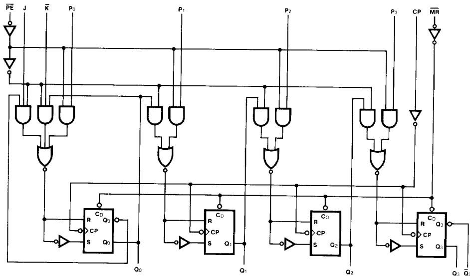
**FUNCTIONAL DESCRIPTION** — The Logic Diagrams and Truth Table indicate the functional characteristics of the '00 4-bit shift register. The device is useful in a wide variety of shifting, counting and storage applications. It performs serial, parallel, serial-to-parallel, or parallel-to-serial data transfers.
