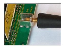
SCRTM4RA is a PCB Mounting terminal which accept any M4 screw thread antenna. For further data please see DS-SCRTM4RA.
