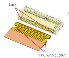
FPC LOCK mechanism maintains high FPC retention force
