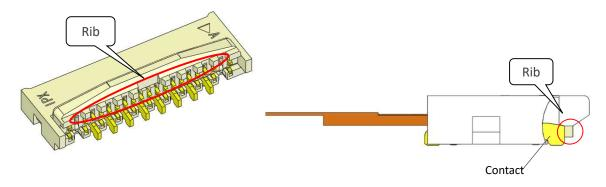
When opening the actuator, the ribs will prevent the contacts from being pulled up.
