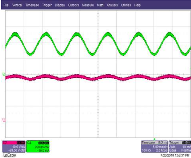
Figure 21 – 90 VAC, Full Load. Upper: I_{RIPPLE} , 0.2 A / div. Lower: V_{OUTPUT} 10 V, 5 ms / div.
