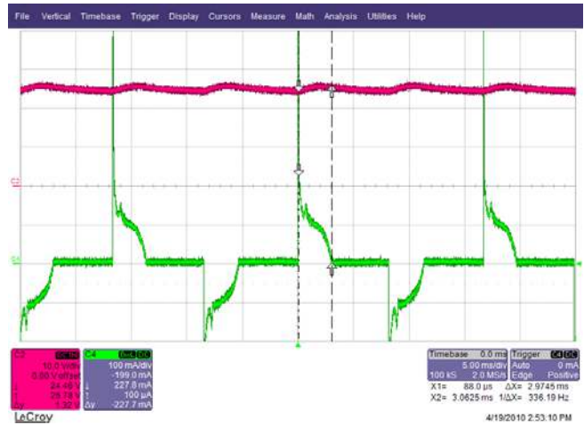
Figure 31 – 115 VAC, 65° Phase. Upper: V_{OUT} , 10 V / div. Lower: I_{IN} , 0.1 A / div., 5 ms / div.
