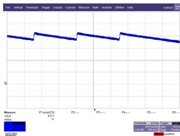
Figure 28 – Output Voltage: 230 VAC. V_{OUT} , 10 V / div., 500 ns / div.
