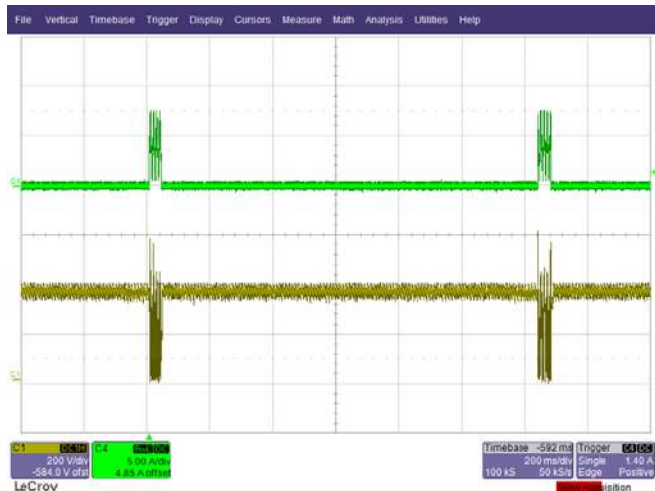
Figure 26 – 265 VAC, Full Load. Upper: I_{OUTPUT} , 5 A / div. Lower: V_{OUTPUT} , 200 V, 200 ns / div.
