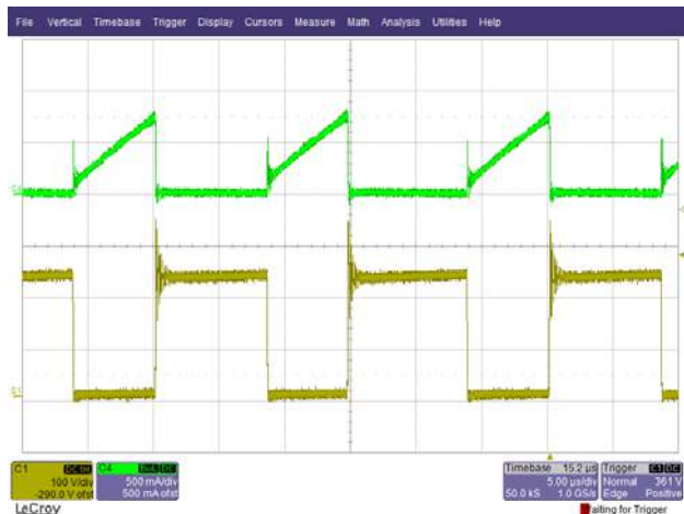
Figure 19 – 90 VAC, Full Load. Upper: I_{DRAIN} , 0.5 A / div. Lower: V_{DRAIN} , 100 V, 5 \mu s / div.
