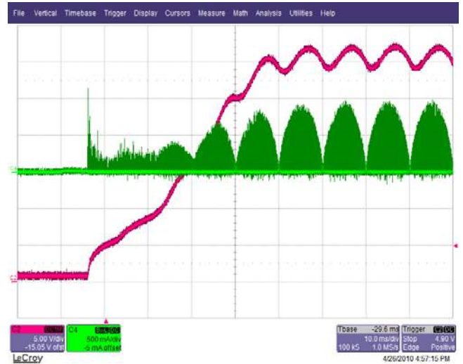
Figure 24 – 265 VAC, Full Load. Upper: I_{RIPPLE} , 0.5 A / div. Lower: V_{OUTPUT} , 5 V, 10 ms / div.
