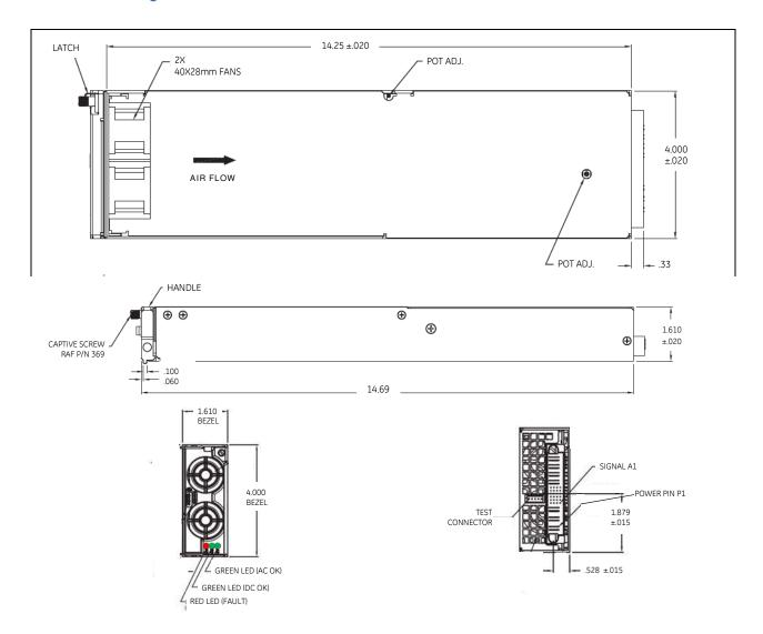
Input: 90Vac to 264Vac; Output: 48Vdc @ 2500W; 3.3Vdc or 5 Vdc @ 1A
