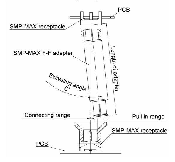
The connecting range represents the maximum misalignment during connection.
