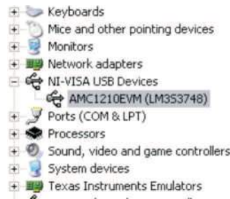
Figure 6. NI-VISA AMC1210MB-EVM Driver Verification
