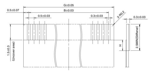
Note 1 : Stiffener dimension should be 2.5mm min., and H dimension should be 0.5mm for improved flexibility of FPC. Note 2 : When using the FPC/FFC in FH34S or FH19SC connectors, the exposed area inserted in either connector is 2.5mm ± 0.3mm and the stiffener is 3.5mm min.
