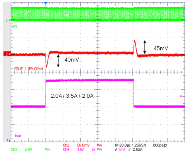
Figure 33. Transient Load 2.0 – 3.5 A Forced PWM Mode
