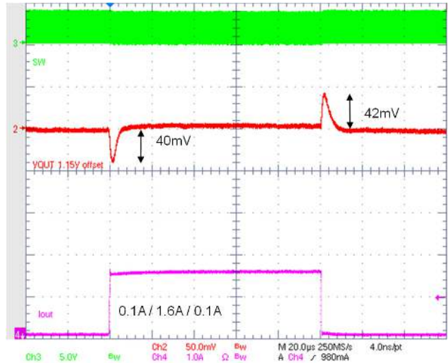
Figure 29. Transient Load 0.1 – 1.6 A Forced PWM Mode
