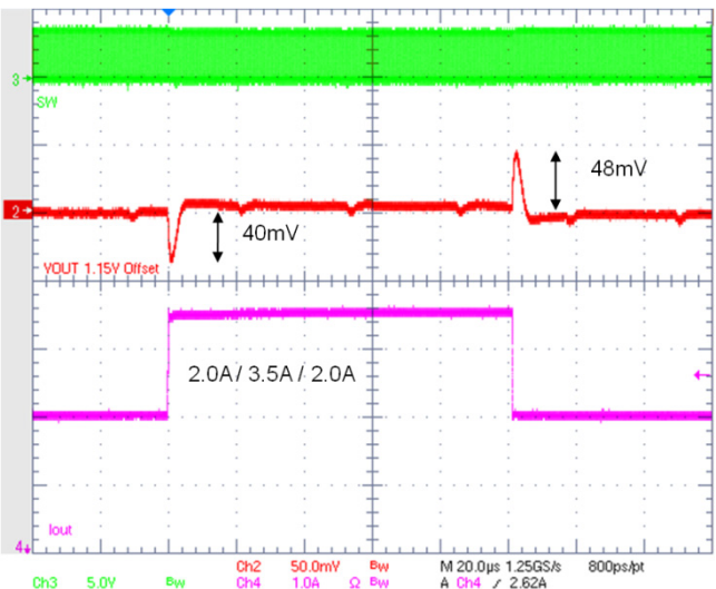
Figure 32. Transient Load 2.0 – 3.5 A Auto Mode
