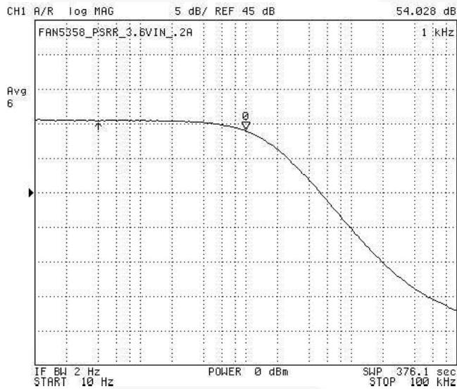
Figure 19. Power Supply Rejection Ratio at 200mA Load
