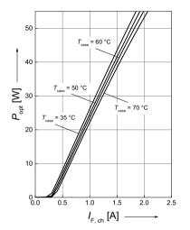
Typical optical output power, cw  $^{2) 3) page 10}$  $P_{opt, package} = f(T_{case}); I_{F, ch} = 2 A$
