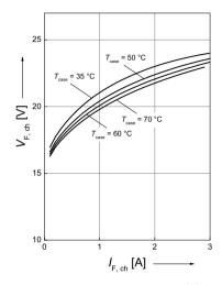
Forward voltage per channel, cw  $^{2) 3)$  page 10  $V_{F, ch} = f (T_{case})$ ;  $I_{F, ch} = 2$  A
