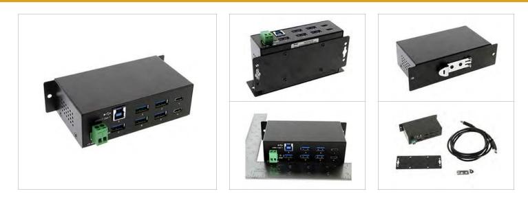
USB 3.1 USB-C hub incorporates 5 USB Type-A and 2 USB-C reversible ports downstream and 1 USB-B Upstream port. This is a great hub choice for applications that need 5Gbps data speeds and multiple mounting options. It is backward compatible with USB 2.0/1.1 compliant host using its RISC-like USB controller. It provides a unique self-power mode to work with wide range (+7 ~ 48V DC) input DC power from its terminal block (power adapter sold separately).
