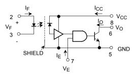
A 0.01 to  $0.1 \mu F$  bypass capacitor must be connected between pins 8 and 5 (see Note 1)
