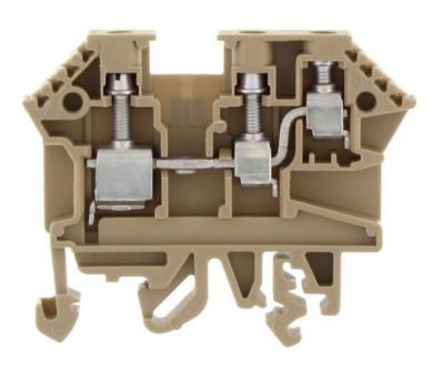
Feed-through terminal, Screw connection, Mounting type:Mounting rail TS 35/7.5 and TS 32, Rated cross-section: 4 mm², Width: 6 mm, Colour: Beige
