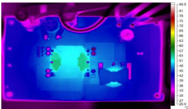
Figure 5. Thermal Map, Front Side at 12V IN and 1.5A OUT (T A = 25°C)
