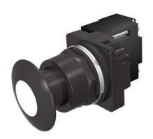
30mm BlackMax, Epoxy Coated Corrosion Resistant Complete Metal Unit Illuminated Push-Pull Operator Transformer type, 480V AC Incandescent Lamp Mushroom Head Cap Small 1 3/4" (44.5 mm) Metal, Black with White Lens 3 Position Momentary UL Listed, CSA Certified NEMA 1,3,3R,4,4X,12,13 & Automotive Standards
