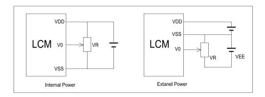
$V_{DD^{\sim}}V_0\text{: LCD Driving voltage}$
