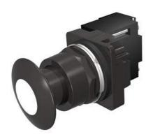
30mm BlackMax, Epoxy Coated Corrosion Resistant Complete Metal Unit Illuminated Push-Pull Operator Full Voltage, 12V AC/DC Incandescent Lamp Mushroom Head Cap Small 1 3/4" (44.5 mm) Metal, Black with White Lens 3 Position Momentary UL Listed, CSA Certified NEMA 1,3,3R,4,4X,12,13 & Automotive Standards
