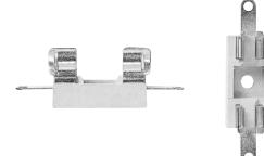
Dimensions (mm) Catalog Symbol: HTC-10M Voltage Rating: 250 Volts Ampere Rating: 6.3 Amperes 4 (± 0.15) 13.5 Base Material: Beige polyphenylene oxide  $(\pm 0.15)$ Flammability: UL 94-V1 Glow Wire Test: 960°C per IEC 695-2-1 Terminals: Tin-plated brass Agency Approvals: 22 (± 0.1) UL Recognized, File No. E19180 Contact Resistance: ≤10 Mohms <u>0</u>.1 × h = 1.5 3.2 Insulation Resistance: ≥10 Mohms Dielectric Strength: ≥2500V ± 0.1 G
