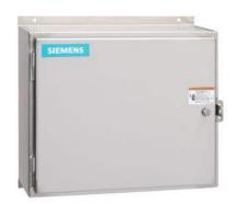
Mechanically held lighting contactor, Contactor amp rating 60Amp 0NC - 10NO poles, 550VAC 50HZ/600VAC 60HZ coil, Non-combination type, Enclosure NEMA type 12, Dust/drip proof for indoors
