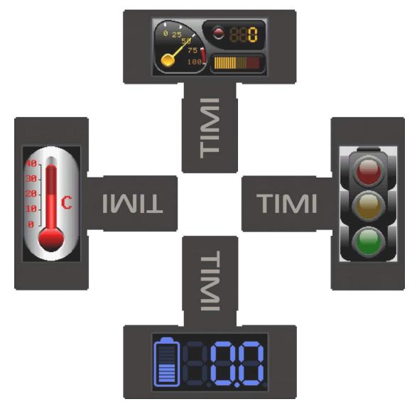
While the TIMI-96 can be orientated in any of its 4 positions, Portrait, Landscape, Portrait Reversed and Landscape Reversed, its natural position forms an upside-down 'T' shape and is designed to interface with the bottom of a breadboard, sitting closest to the User, leaving the top part of the breadboard free for components and wiring.
