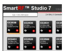
After installing the tool, connect the EB to the PC using the USB cable and start SmartRF Studio. Select the "2.4 GHz" tab and click the refresh ("Find device") button in the lower right corner. Studio will now find the connected SmartRF06EB. Double click on the detected SmartRF06EB to launch the CC2538 device control panel.
