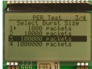
On the transmitter, select the desired burst size, that is, the number of packets to transmit.
