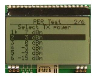
On the transmitter, select desired output power.
