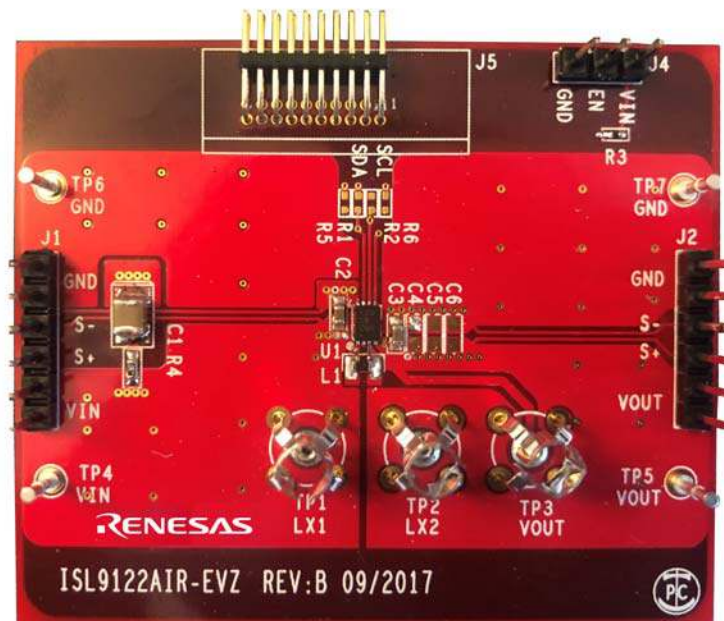
Figure 6. ISL9122AIRN-EVZ Evaluation Board (Top)
