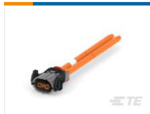
TE Part # 1-2286937-6 2POS,HVP800,180 DEG,50 SQMM, COD A,CS
