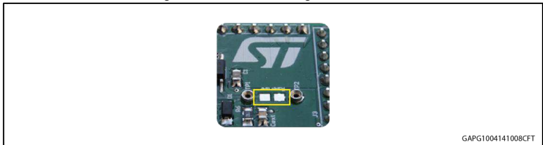
Figure 5: Pads for soldering SMD resistor
