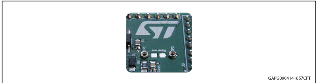
Figure 4: Mounting through-hole sense resistor
