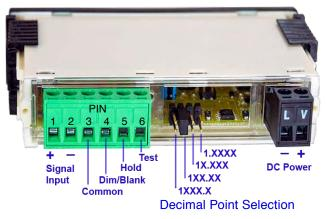
**Display Test:** All numeric display segments will light up when Display Test Pin 6 is connected to Common Pin 3.
