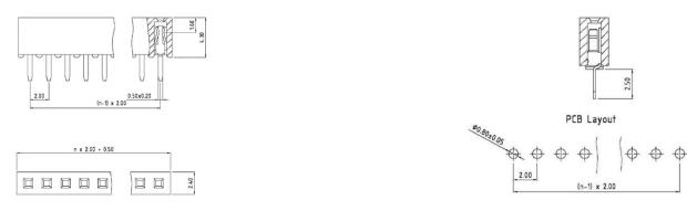
When using the recommended connector, ensure that any baseboard components placed under the Skywire (between the header connectors) are shorter than 4 mm. However, the max component height may change depending on the chosen connector.
