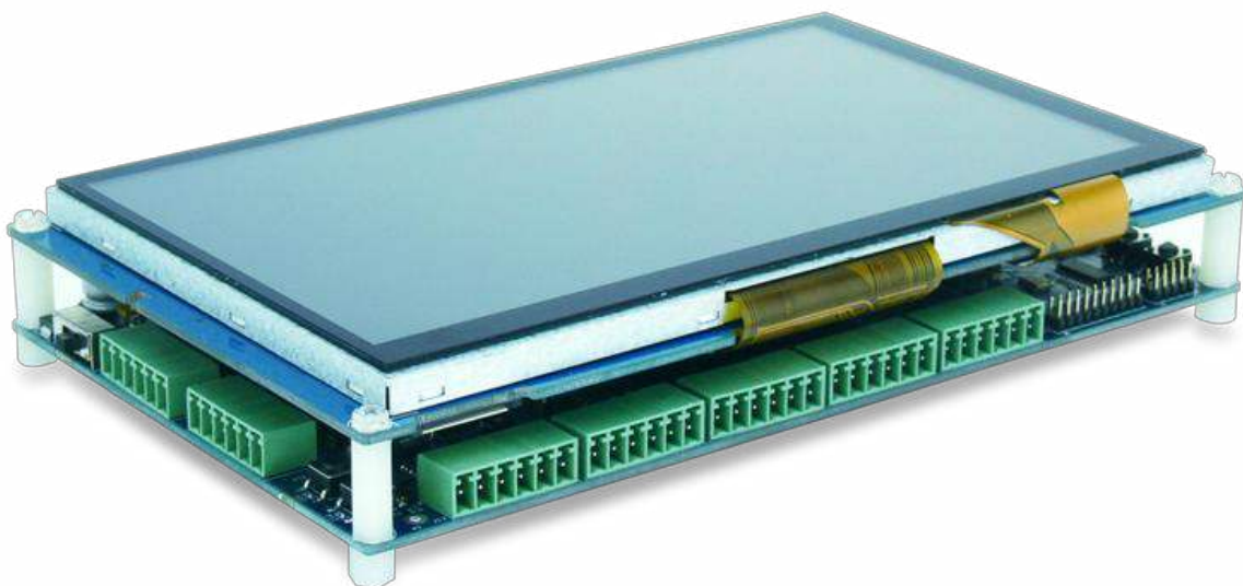
MYD-AM335X-J Development Board with 7-inch LCD Module
