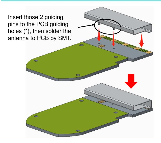
\* The 2 guiding holes on PCB must be non plated holes without any metal.
