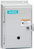
Non-reversing contactor, Size 1 3/4, Three phase full voltage, Contactor amp rating 40A, 3 wire (NO aux included), 220-240/440-480VAC 60Hz coil, Non-combination type, Enclosure NEMA type 12, Dust/drip proof for indoors, Extra-wide enclosure
