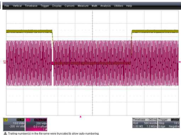
CH1:Vo (10 V/div) CH2:Vin (200 V/div) Figure 12: AC drop out 50 mS@230 VAC (50 mS/div), Vo restart
