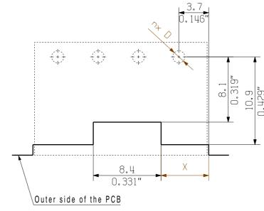
Hole pattern using MPS 5 with middle flange lever
