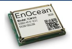
The serial interface operates according to EnOcean ESP3 standard with the option to use higher interface speeds (TURBO mode) to reduce latencies.
