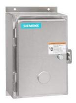
Non-reversing NEMA contactor, Size 0, 4 power poles, Contactor amp rating 18A, 3 wire (NO aux included), 110V 50Hz / 120V 60Hz coil, Non-combination type, Encl NEMA type 4X 304 S-Steel, Water/dust tight noncorrosive, Standard width enclosure
