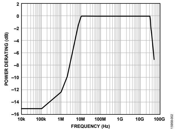
Figure 2. Power Derating vs. Frequency, Low Frequency Detail, T_{CASE} = 85^{\circ}C
