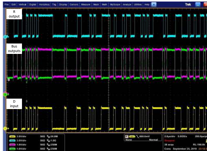
Figure 22. Waveforms at 10 Mbps Operation, PRBS7 Data Pattern
