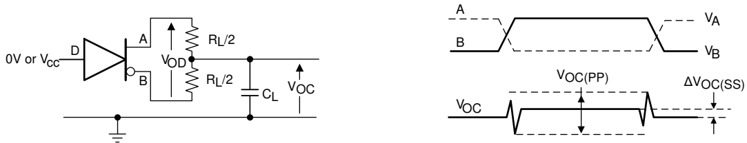
Figure 8. Measurement of Driver Differential and Common-Mode Output With RS-485 Load
