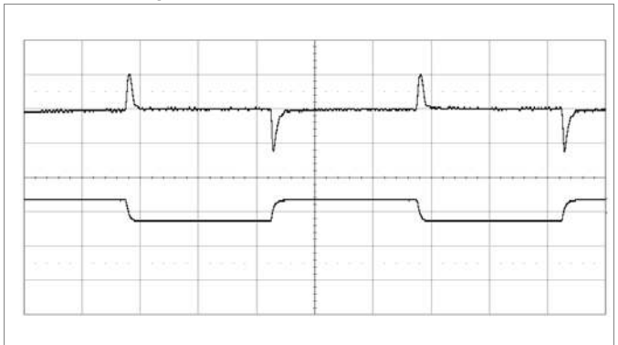
Output voltage response to load current step change (1.5-4.5-1.5 A) at V_i = 12\text{ V} , C_o = 3 \times 100\ \mu\text{F} + 270\ \mu\text{F}/10\text{m}\Omega . Default compensation settings. Scale: 20 mV/div, 5 A/div, 100 \mu\text{s} /div.
