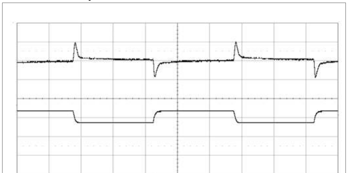
Output voltage response to load current step change (1.5–4.5–1.5 A) at V_I = 12\text{ V} , C_O = 3 \times 100\ \mu\text{F} + 270\ \mu\text{F}/10\text{m}\Omega . Default compensation settings. Scale: 20 mV/div, 5 A/div, 100 \mu\text{s} /div.
