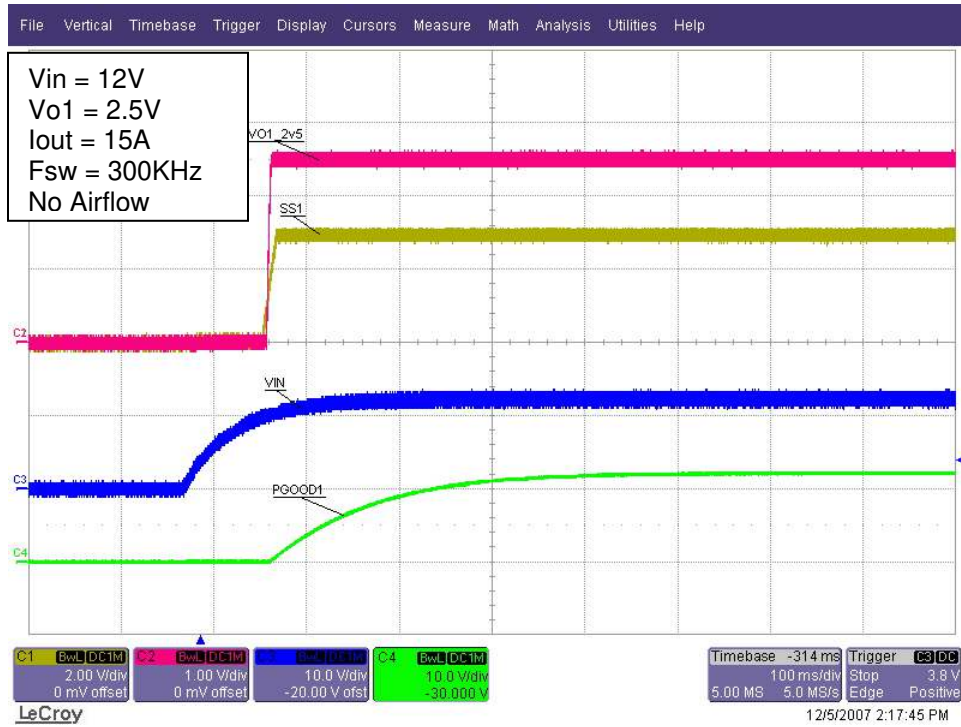
Fig.7: Vo1 Power Up Sequence
