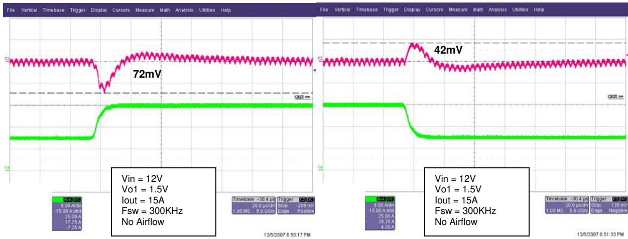
Fig. 21: I_{out2} Transient Step-Up 50% - 100%
