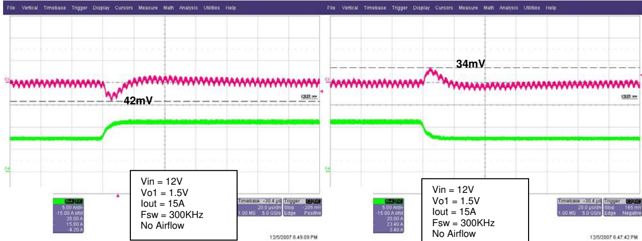
Fig. 19: I_{out2} Transient Step-Up 50% - 75%
