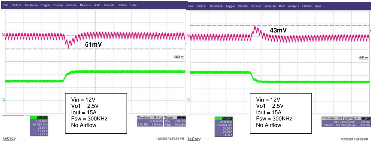
Fig. 15: I_{out1} Transient Step-Up 50% - 75%
