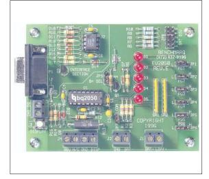
The menu-driven software provided with the EV2050 displays charge/discharge activity and allows user interface to the bq2050 from any standard DOS PC.
