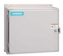
Mechanically held lighting contactor, Contactor amp rating 60Amp 0NC  $\_$  9NO poles, 277VAC 60HZ coil, Non-combination type, Enclosure NEMA type 12, Dust/drip proof for indoors
