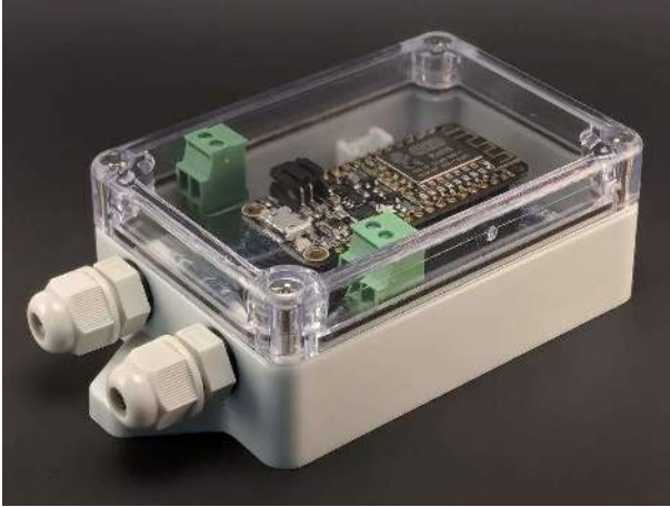
Pic.8. qBoxMini Enclosure Plus Kit with Adafruit Feather Compatible board installed
