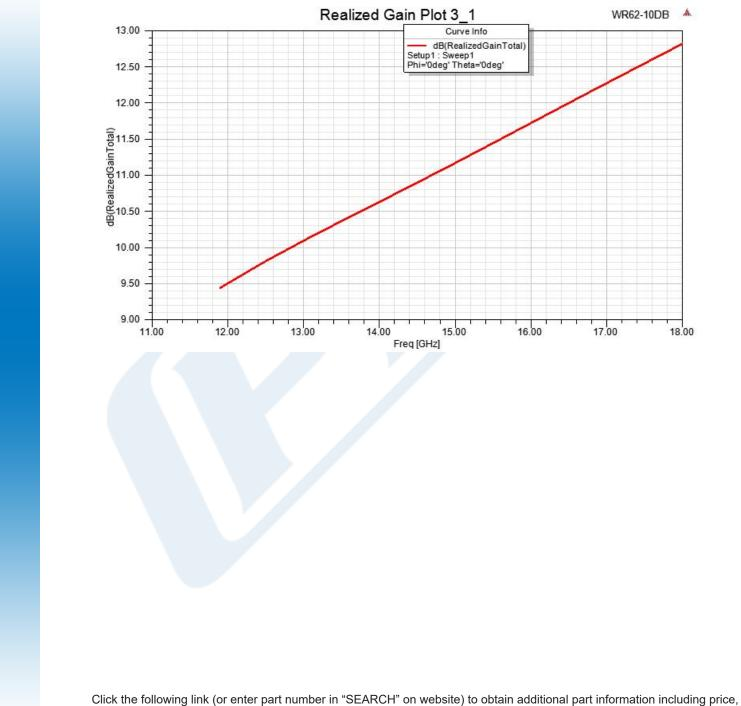
inventory and certifications: WR-62 Standard Gain Horn with 10 dBi gain, SMA Male connector PEWAN062-10SM
