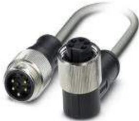
Bus system cable, DeviceNet, 5-position, PUR halogen-free, Gray RAL 7001, Plug straight 7/8"-16UNF, on Socket angled 7/8"-16UNF, Cable length: 0.3 m
