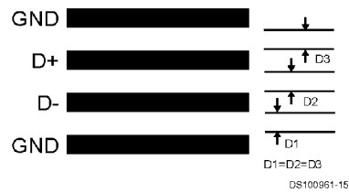
FIGURE 6. Recommended Diode Trace Layout
