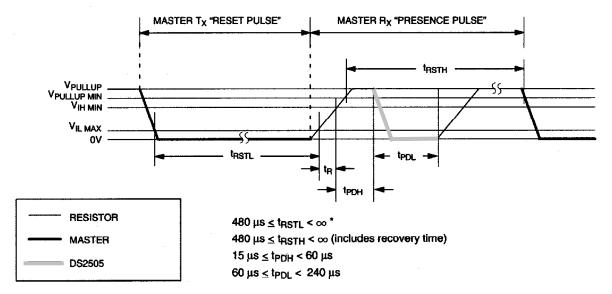
\* In order not to mask interrupt signaling by other devices on the 1-Wire bus,  $t_{RSTL} + t_R$  should always be less than 960 µs.
