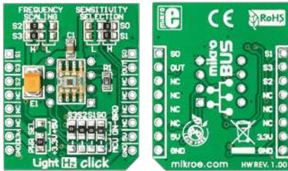
Front and back side appearance of the LightHz click Board
