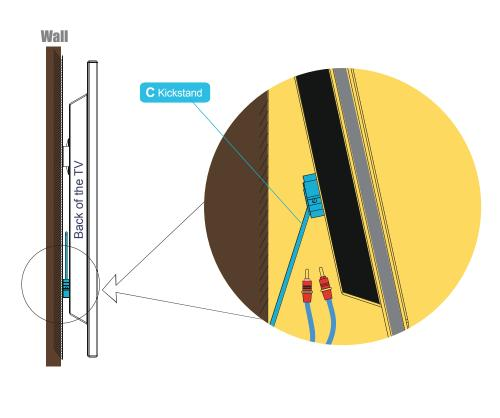
Fold out the kickstands to access the cables behind the TV. Once all cables are installed, unfold the kickstands.
