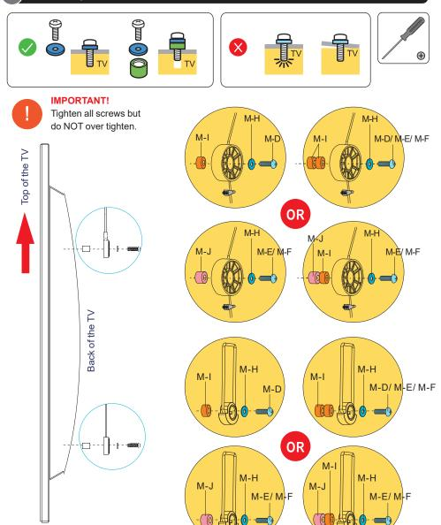
Choose the appropriate screws, washers, and spacers (if necessary) according to the type of your TV and tighten the adapter brackets (B) and the kickstands (C) to the back of the TV using a Philips screw driver.
