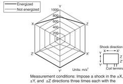
Relay energized to check the shock values that cause the Relay to malfunction.
