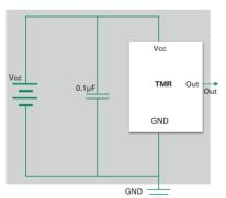
Note: It is strongly recommended that an external bypass capacitor be connected in-close-proximity to the device between the supply and ground pins to reduce noise. The recommended value for the external bypass capacitor is  $0.1\mu F$ .
