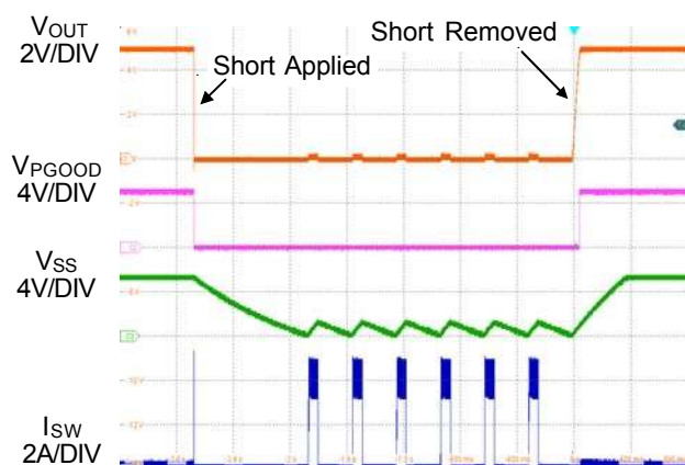
Figure 3. Short Circuit Protection and Recovery
